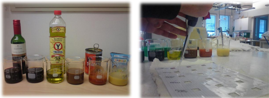
Image 4-1: The left panel shows soil substances used in the test and the right panel shows stain application.
