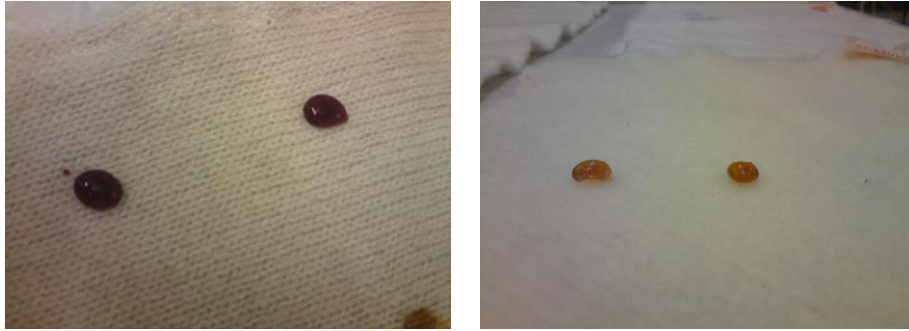
Image 4-3: The left panel shows red wine droplets on knitted wool and the right panel shows coffee droplets on woven wool
