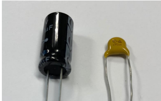
Figure 15: Electrolytic capacitor (left) and ceramic capacitor (right)
