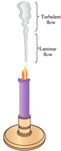
Figure 3: Flow regimes of a candle smoke plume [3]
