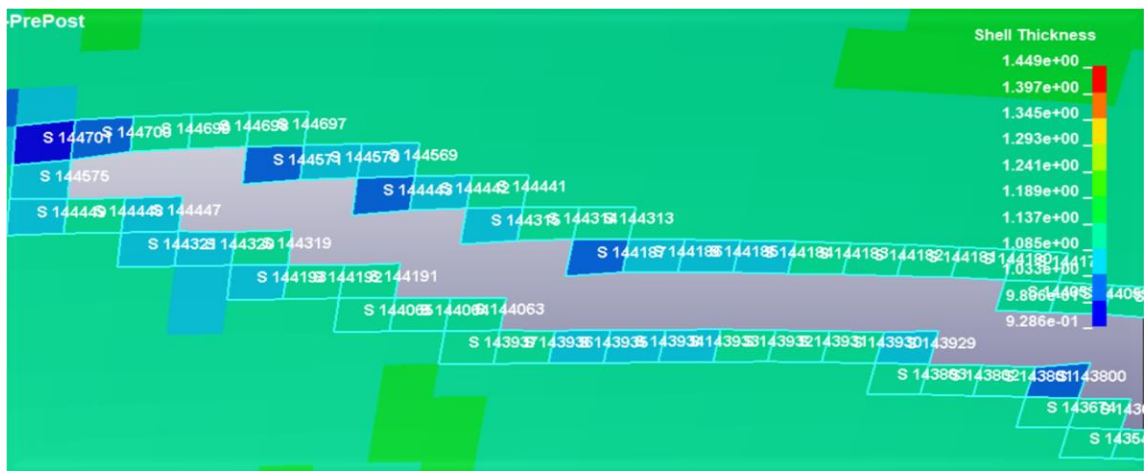
Figure 25: The location of fracture resulting from a randomly distributed shell thickness
