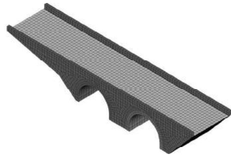
Fig. 6 3D FE mesh of Roman Bridge.
