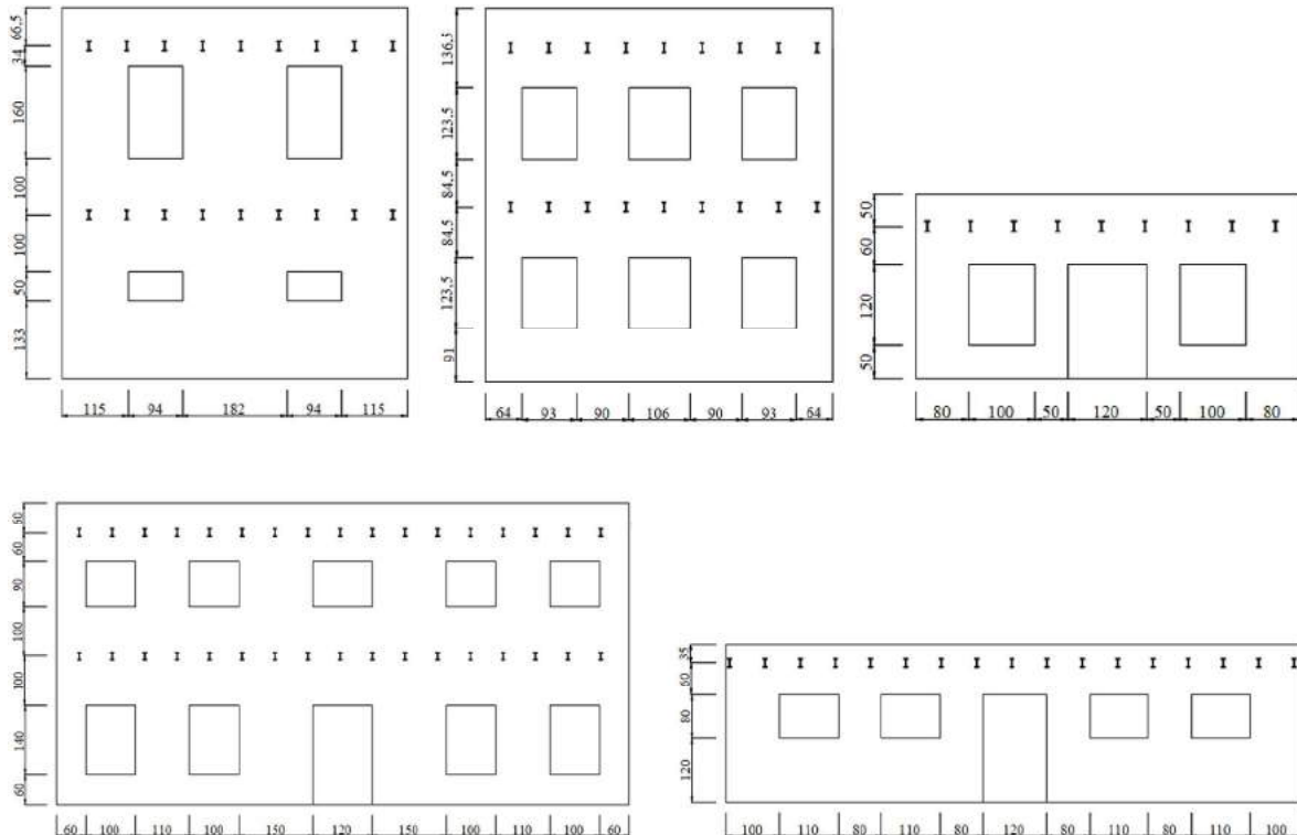
Fig. 5. Added five case studies chosen for the evaluation of the zero-moment coefficient factor.
