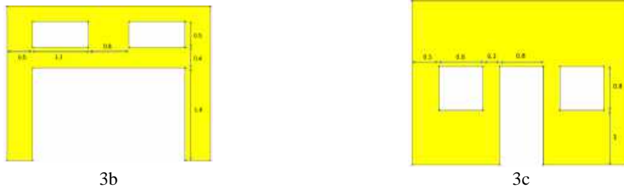
Fig. 3 – Geometry and opening configurations of the URM wall case studies (Dimensions in m).
