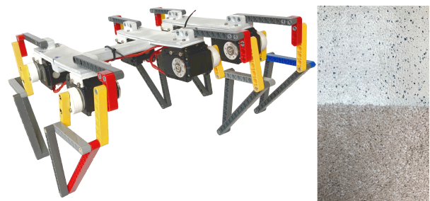
Fig. 2. The hexapod robot platform used for testing the evolved mechanical linkages, and the two floor textures it is tested on.
