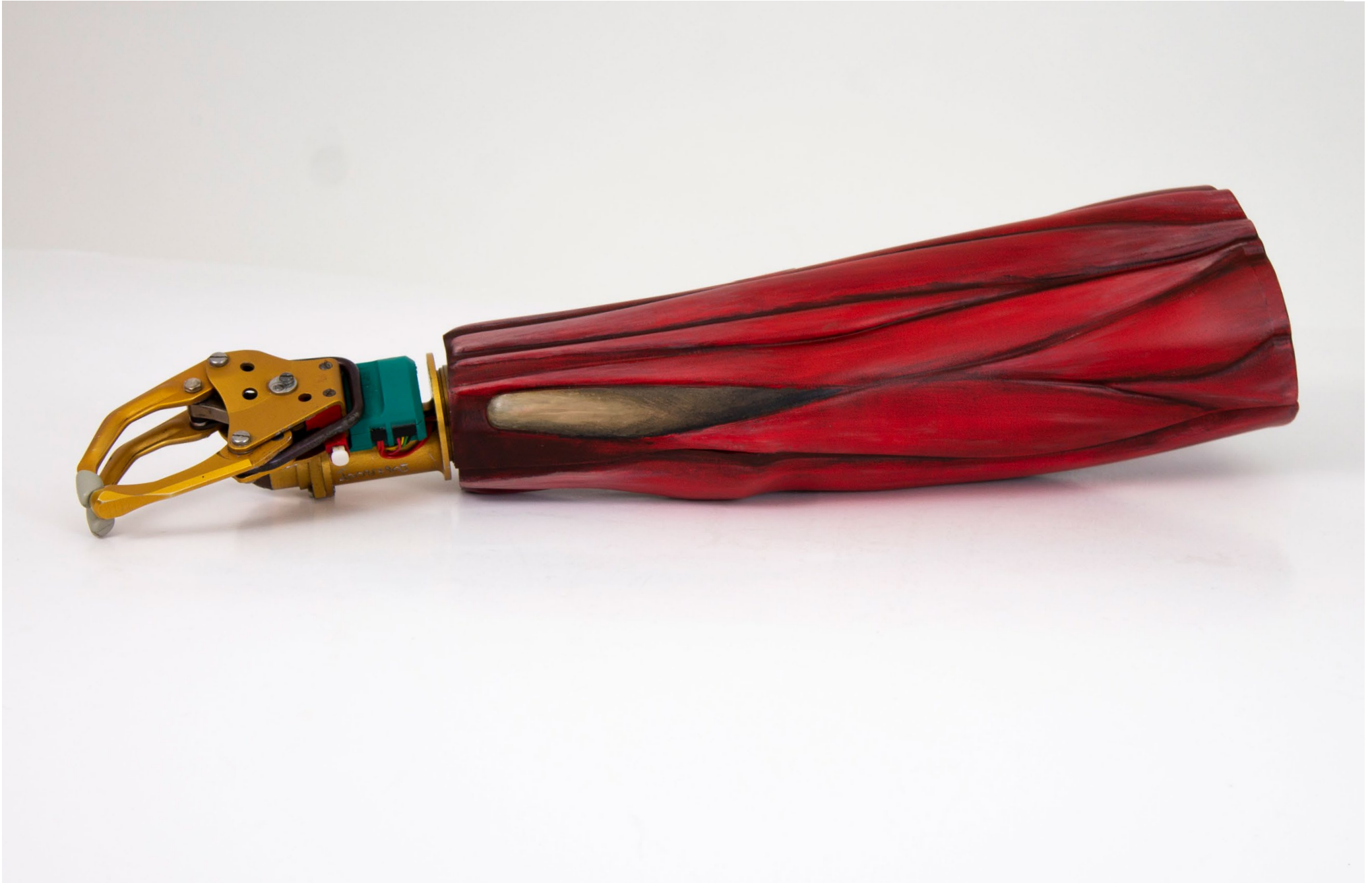
Final prototype. 3D-printed (PLA) and painted. Basic myoelectric hand for illustrative purposes.
