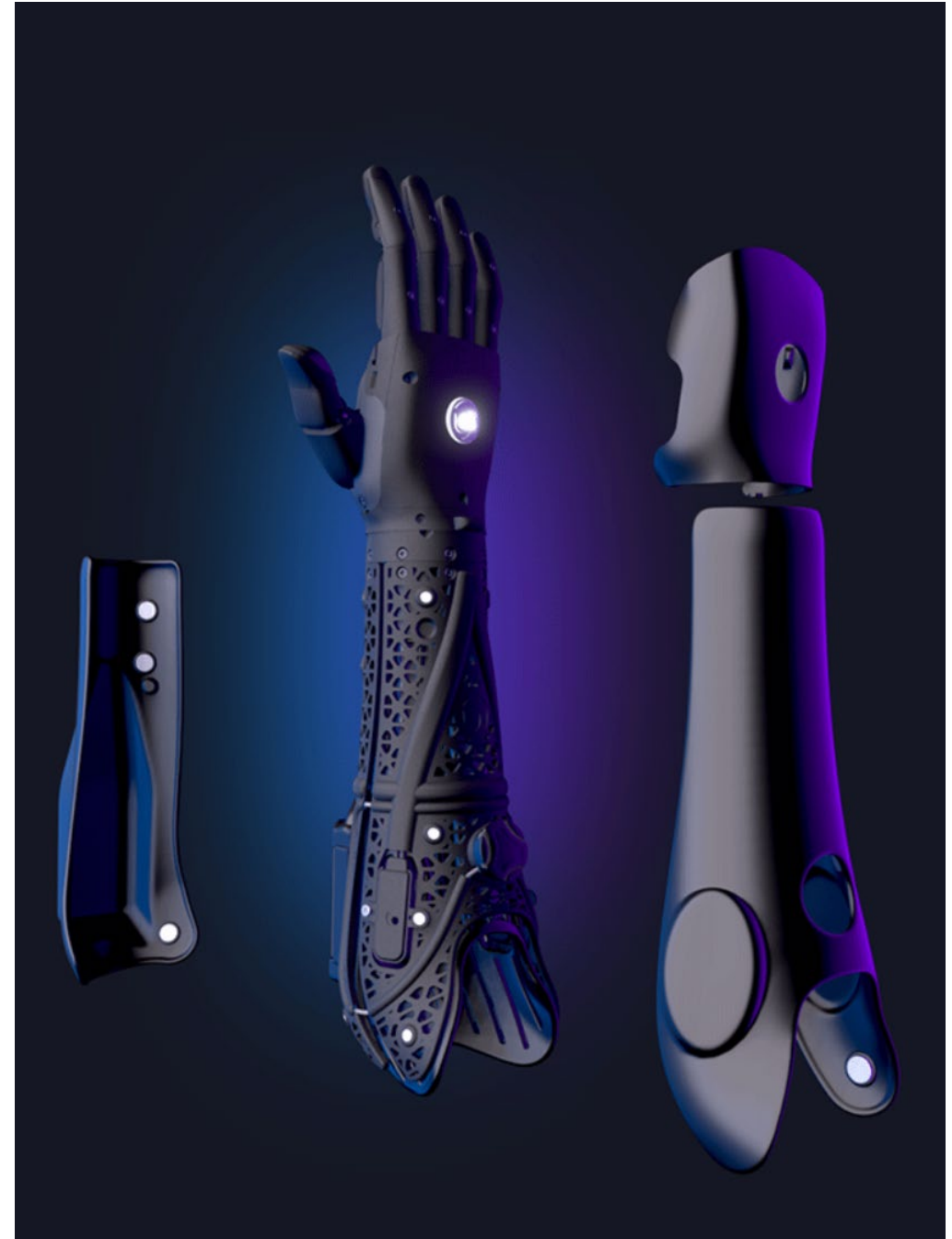
Fig 3. MagSwap™ Removable Covers, retrieved 21.05.2023, by Open Bionics. ( https://openbionics.com/hero-arm-overview/ ).
