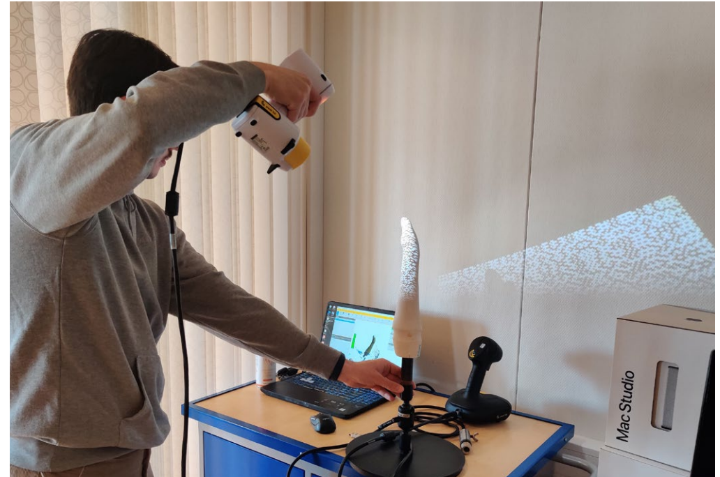
3D-scanning plaster cast of Erik's stump.
