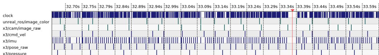
Figure 2.10: Synchronization issue as seen in Rqt Bag. Blue vertical lines indicate when the message is published to ROS. The red line highlights a section where the clock cycle is not published at a regular interval.
