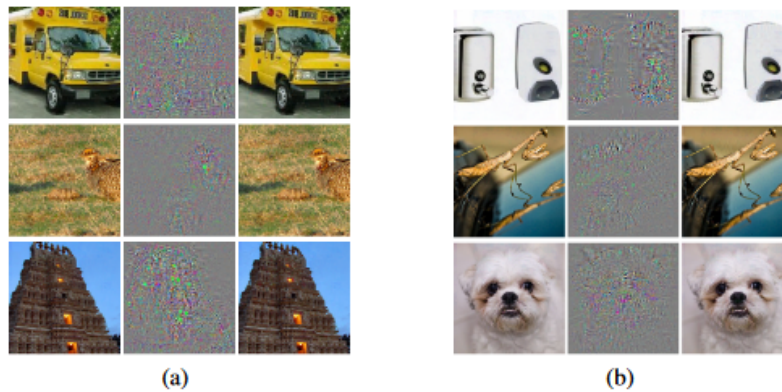
Figure 2.1: Images on the left are the original images with their correct classification, while images on the right are the adversarial examples classified as an ostrich. The noise in the middle is the adversarial perturbations with a magnitude of 10 for visibility. The image is from a research paper by Szegedy et al. [1]
