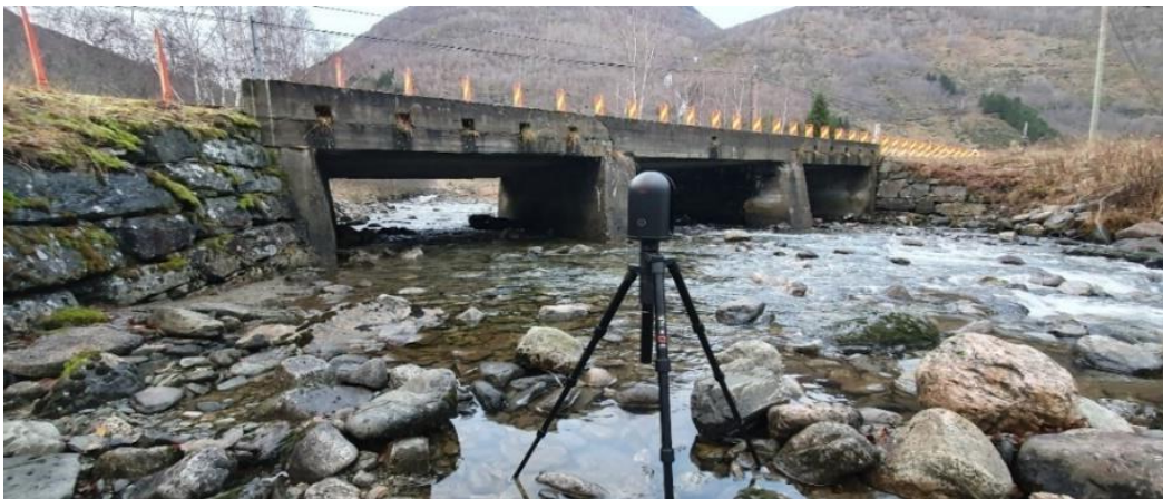
Figure 38: In situ 3D laser scan with Leica BLK360
