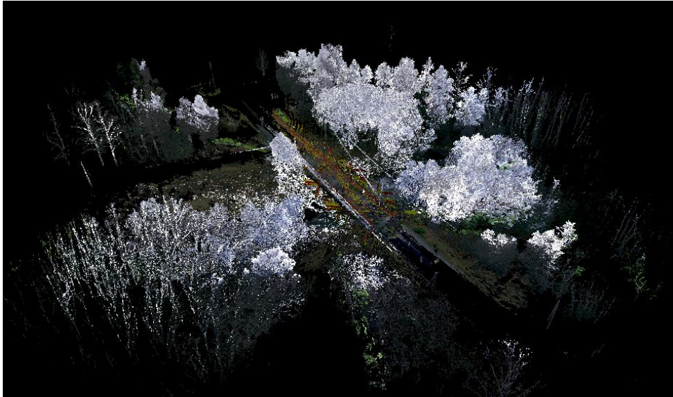
Figure 44: Point cloud generated from all the scans
