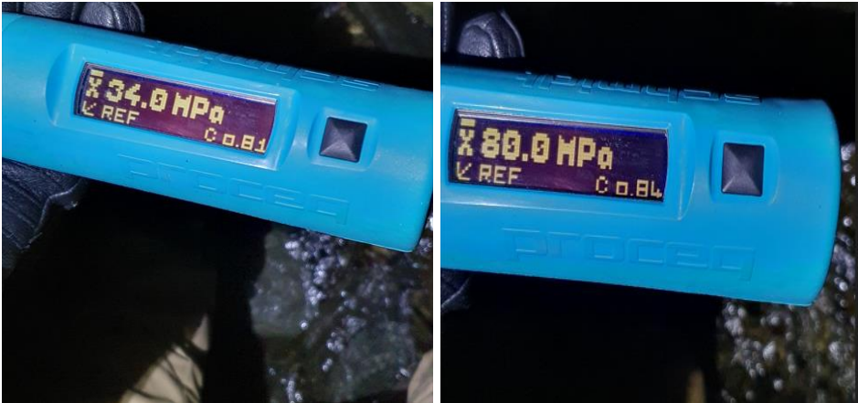
Figure 25: Lowest and highest recorded compressive strength
