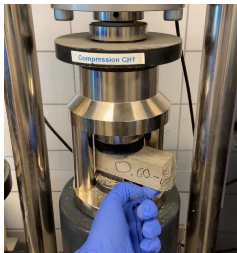
Figure 3.10 Compressive strength test
