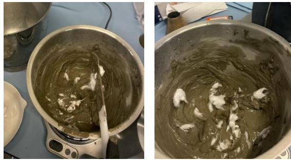
Figure 7-2. Admixture Cement/Microfiber demonstration
