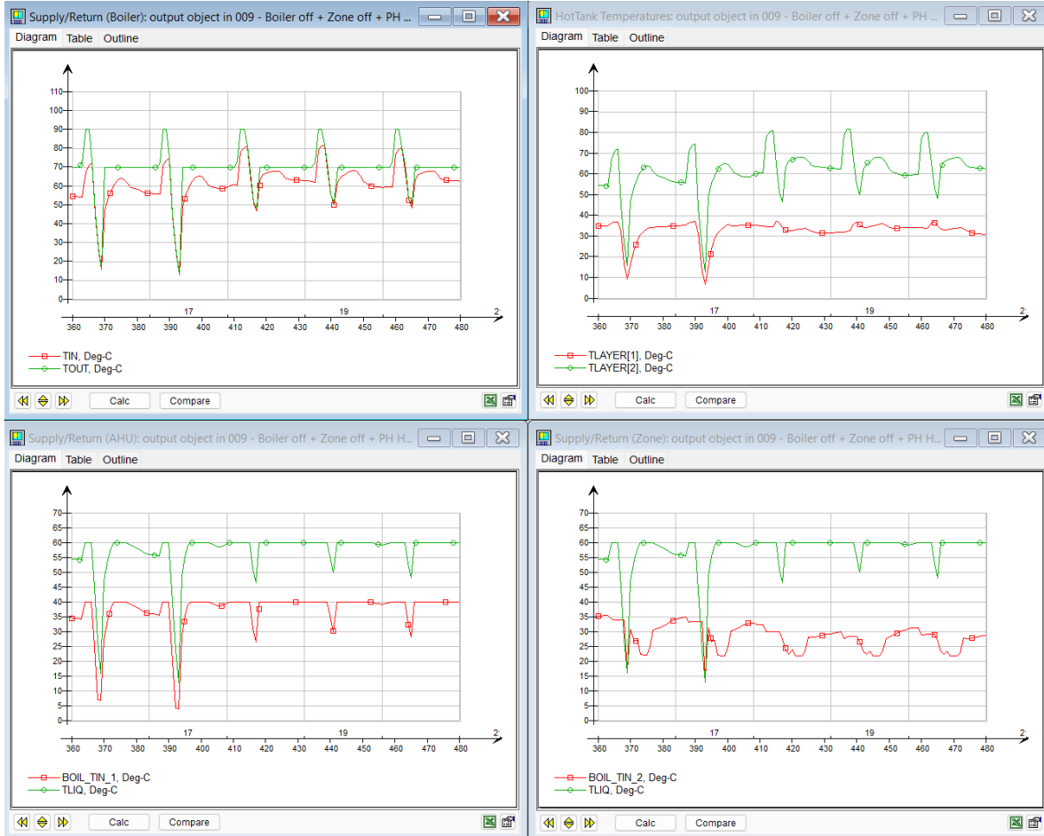
Figure 103: TEK17 case - Simulation 5B. From left to right, top to bottom: Supply/Return temperatures for boiler circuit, Temperature of top and bottom layer of HotTank, Supply/Return temperatures for AHU circuit, Supply/Return temperatures for Zone heating circuit
