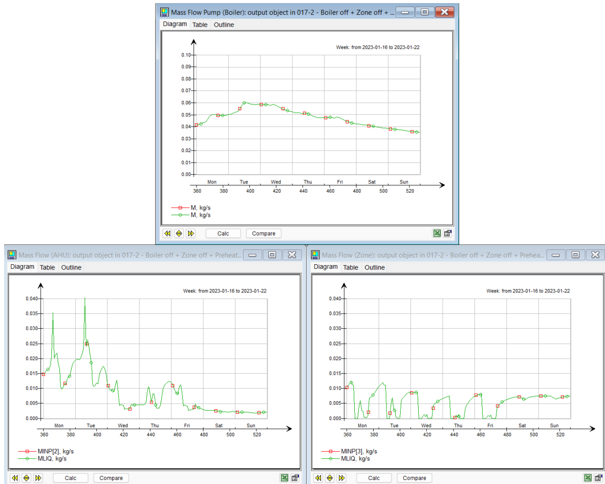
Figure 59: Mass flow rates for PH case - Simulation 4. From top to bottom, left to right: Mass flow of main pump, mass flow of AHU pump, mass flow of zone pump
