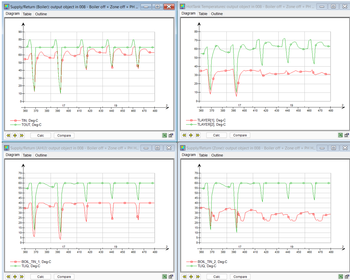
Figure 68: TEK17 case - Simulation 5A. From left to right, top to bottom: Supply/Return temperatures for boiler circuit, Temperature of top and bottom layer of HotTank, Supply/Return temperatures for AHU circuit, Supply/Return temperatures for Zone heating circuit
