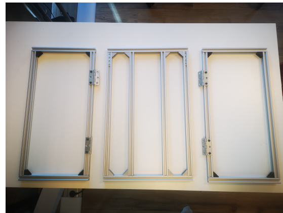
Figure 6.14: Assembled frames with hinges
