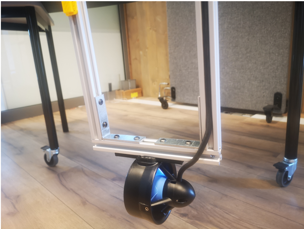
Figure 6.21: Fastening of thruster and cables
