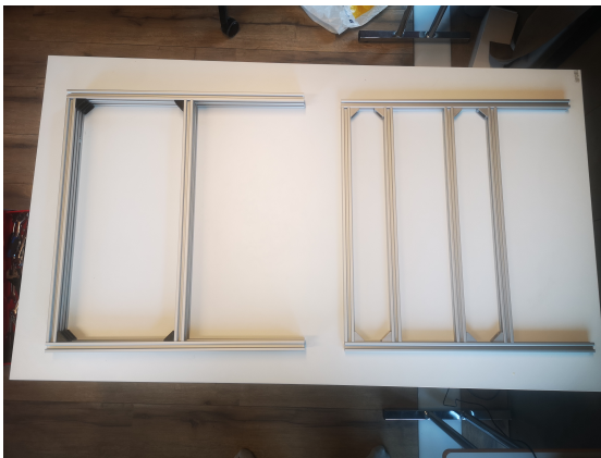
Figure 6.13: Assembling the main- and side frames
