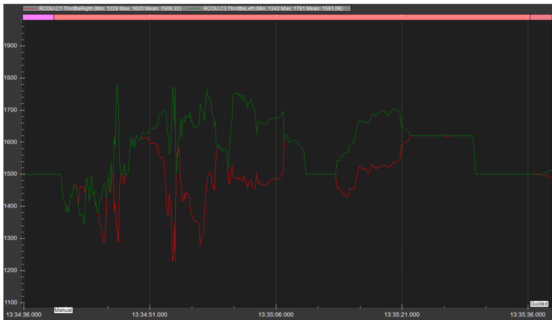
Figure 7.10: Throttle performance during Manual, where throttle right is displayed in red, and throttle left is displayed in green
