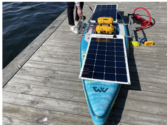
Figure 7.5: Strapping the solar panels to the hull
