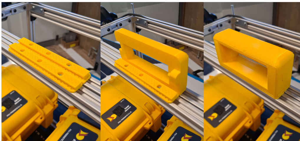
Figure 6.17: Fastening mechanism of the handles
