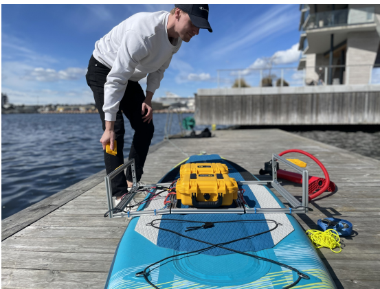
Figure 7.4: Opening and strapping the frame to the SUP board
