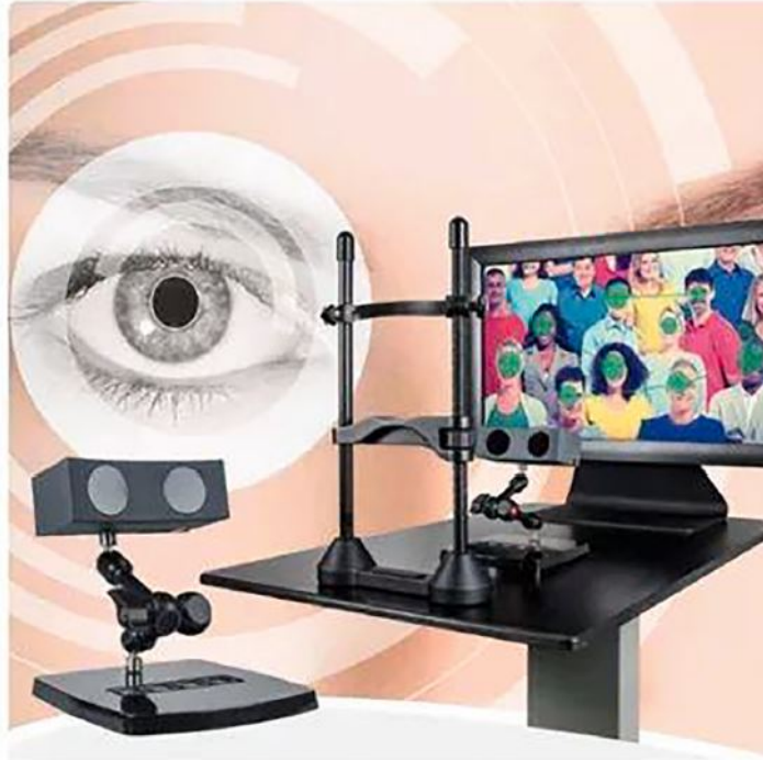
Figure 2.14: Video oculography using two cameras, taken from [73].
