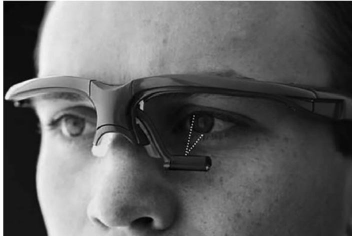
Figure 2.13: Infrared oculography approach setup, taken from [73].
