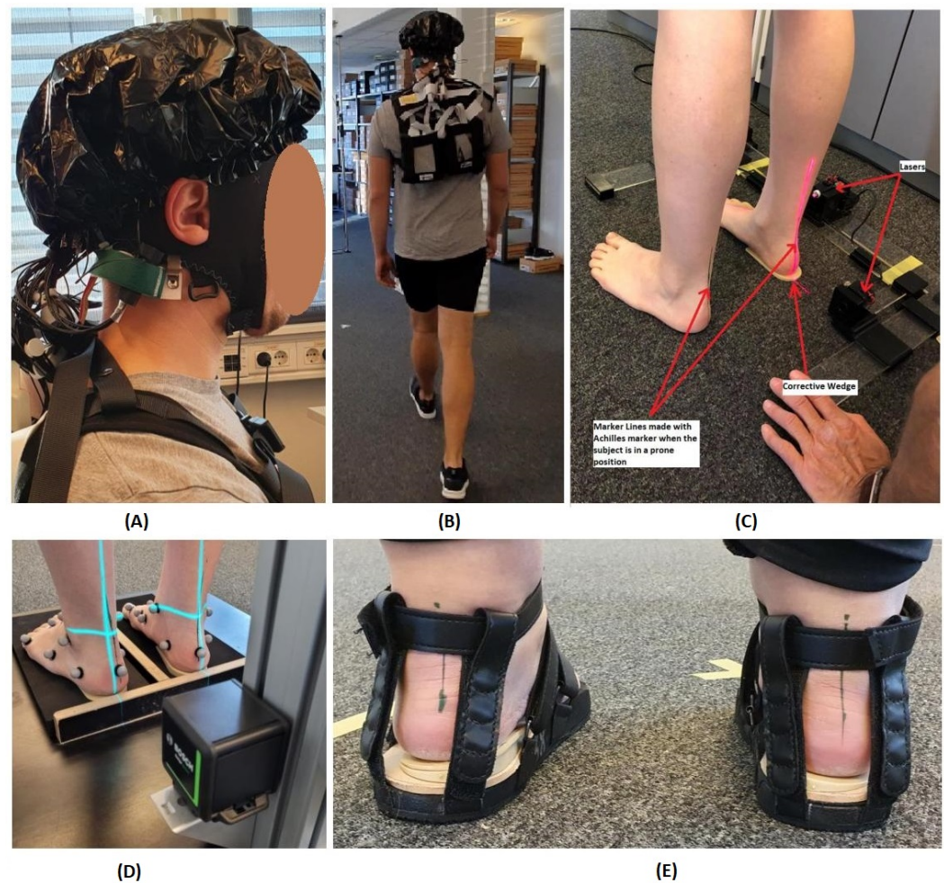
Figure 1. Experimental setup: (A) fNIRS optodes covered with a shower cap to reduce environmental light; (B) demonstration of the subjects performing Infinity Walk with fNIRS equipment; (C) Achilles laser correction line setup; (D) medial wedge correction in posture correction equipment; (E) flat-insole sandal with additional medial wedges to correct the posture.
