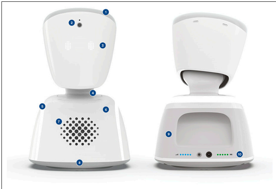
Figure 1. AV1's features. Picture and description from No Isolation's web site: '1. When the student "raises their hand," the top light flashes. 2. A live feed from the classroom is streamed through the microphone and the camera. 3. Student uses the eyes to express emotions. 4. A motor in the neck lets the head turn 80° up and down and side to side. 5. The light strip signals if AV1 is connected or not. 6. The robot has an integrated 4G sim so it is always online. 7. The student's voice is heard from the speaker. 8. A motor at the bottom allows the robot to turn 360°. 9. TPE coated backside that provides great grip. 10. On the back, there is a charger input, battery level indicator, and network quality indicator. 11. AV1 is durable and transportable. It has a hard outer shell'. (No Isolation, NA).
