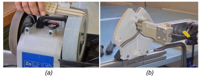
Fig. 3. Sharpening of the smart knife using (a) grinding wheel (T-8, Tormek, Sweden) and (b) straightening tool (ERGO steel III, Bokken AS, Norway).
