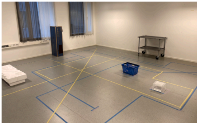
Fig. 3. A photo of the room showing navigation tracks and obstacles. Two tracks were created (refer to Fig. 2). Tapes in two different colors (yellow and blue) were used to indicate the navigation path. The two tracks were made in both directions, resulting in four tracks.
