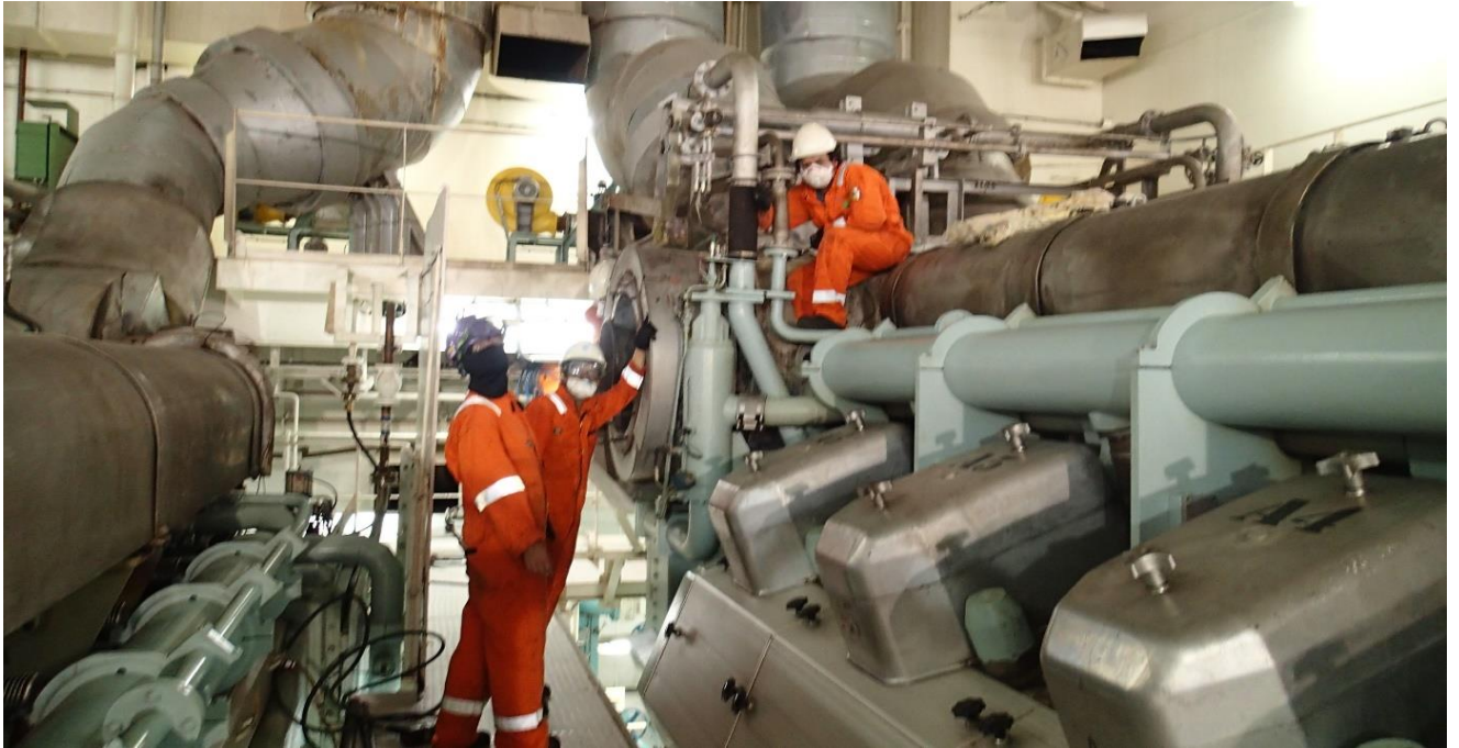
Maintenance work on one of the vessel's four main engines. Photo by author.
