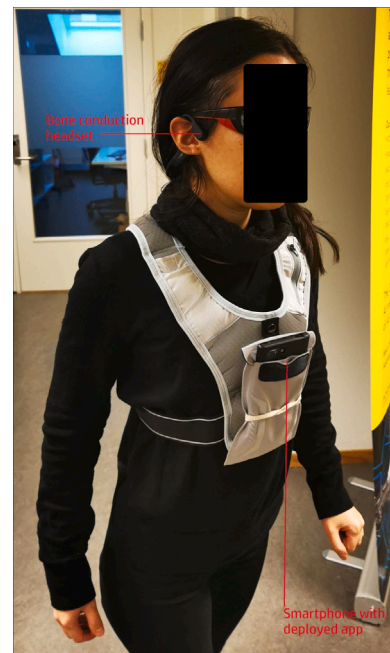
Fig. 10. User testing setup of the navigation assistant. The app is deployed in the smartphone and is placed in the vest where the camera is facing outwards. The user has a bone conduction headset for receiving audio instructions.
