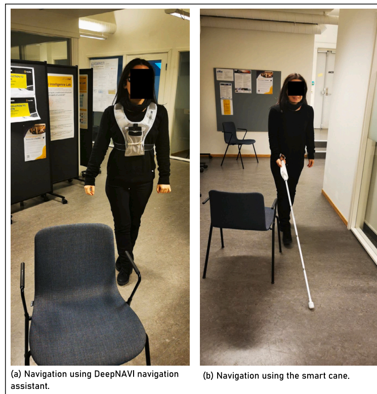
Fig. 11. Photos of the participant navigating with DeepNAVI navigation assistant and smart cane.
