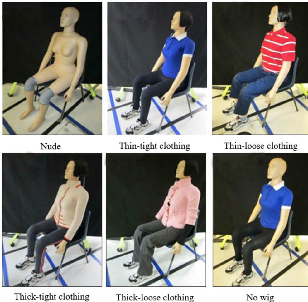
Figure 6. Thermal manikin with different levels of clothing insulation/design. 42
