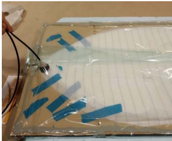
Fig. 4. Hull lid manufactured from fiber glass by vacuum infusion technique
