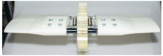
Fig. 12. Dummy test section of wing mounting
