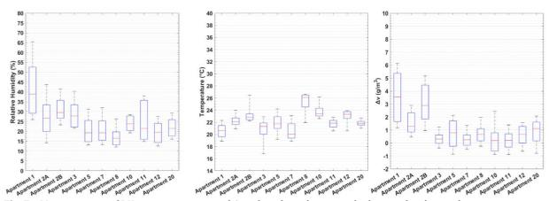
Fig. 7 – Measurements of RH, air temperature and  $\Delta v$  values from the master bedroom of each tested apartment.
