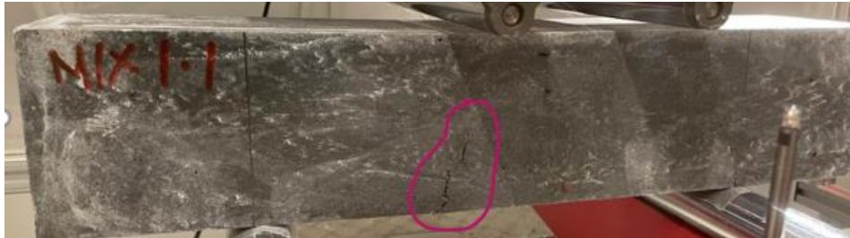
Figure 5.19:Initiation of the crack in beam (Mix I with 2.5% steel fibers)
