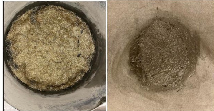
Figure 4.23: Mix with 4% steel fiber (the highest dosage of steel fiber considered in the study)
