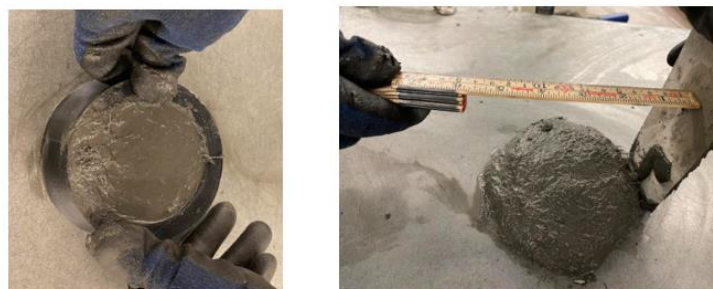
Figure 4.24: flow test done for Mix I
