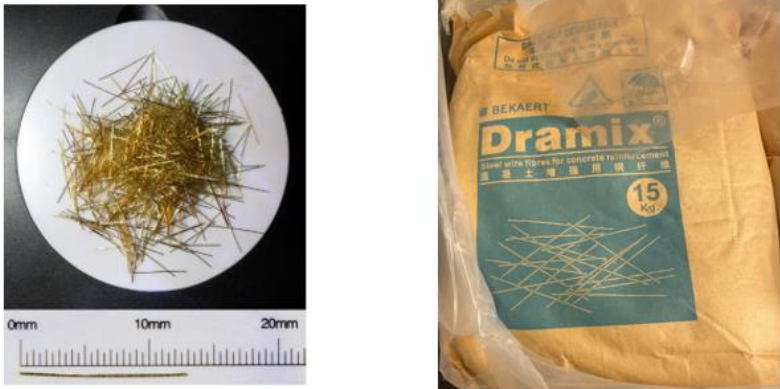
Figure 4.7:Dramix OL 13/.20 steel fiber from Bekaert
