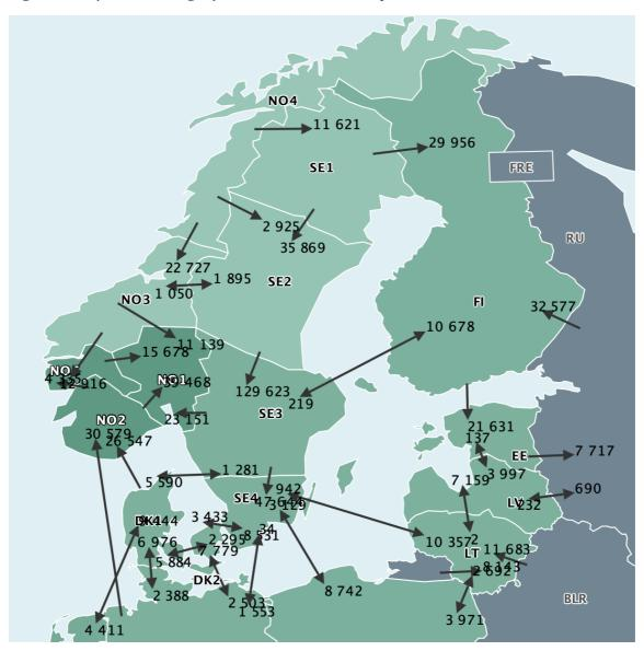
Figure 2.2 Physical Exchange of Power in Northern Europe
