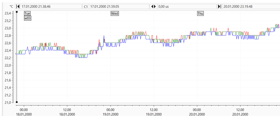
(b) Measured air temperature in hot room
