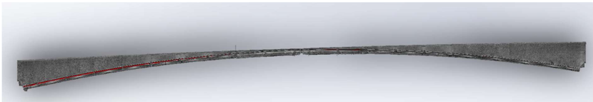
Figure 26: The modelled arch (red) is compared to the point cloud arch
