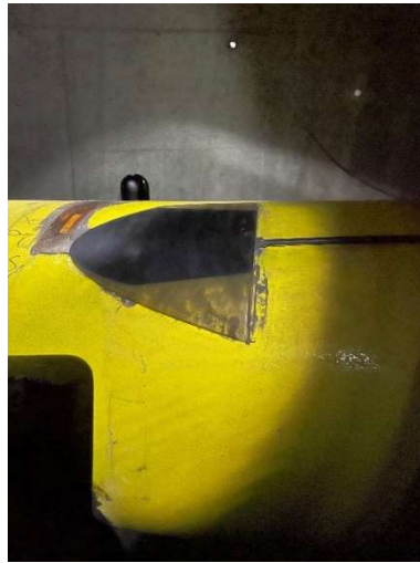
Figure 33: FBG Sensor placed on the arch
