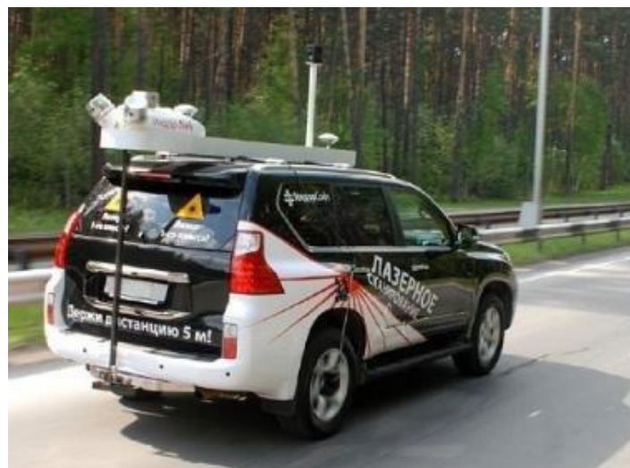
Figure 2.7: Mobile Laser Scanner mounted on a car[24]
