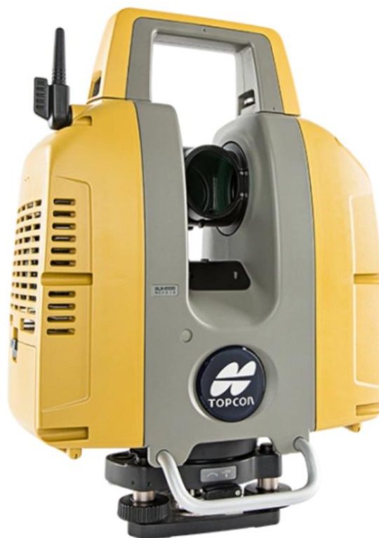
Figure 4.1: Topcon GLS 2000 laser scanner [41]
