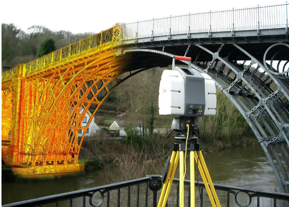
Figure 2.8: Terrestrial Laser Scanning[26]
