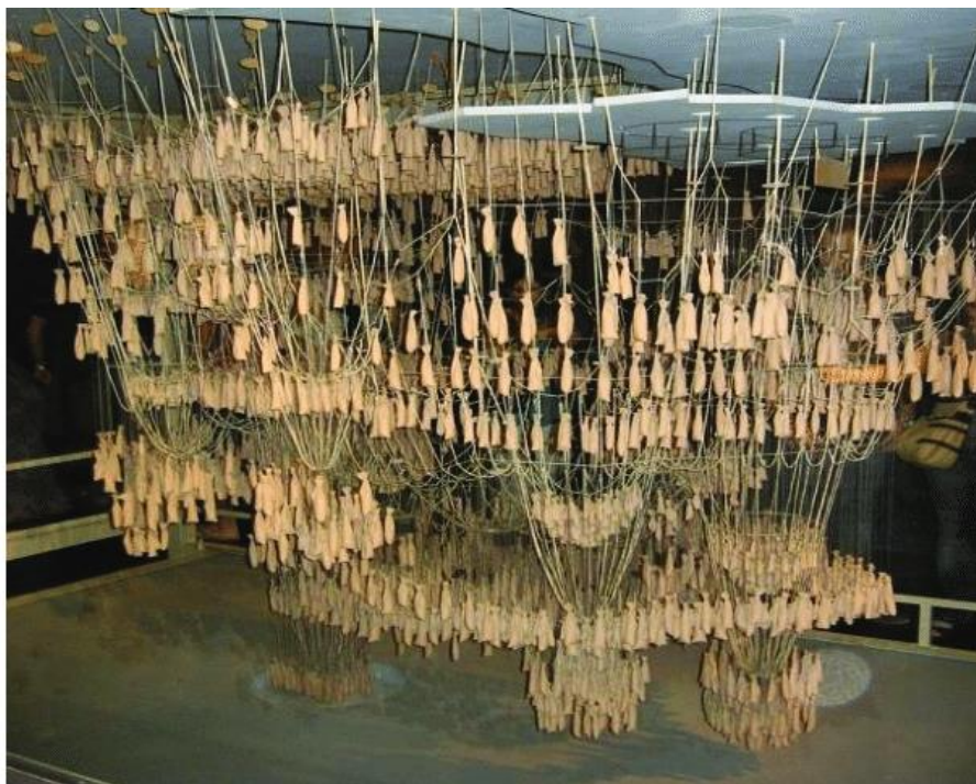
Figure 2.2: An upside-down model of the Church of Colònia Güell [9].
