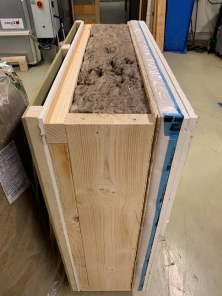
Figure 12: Element filled with mineral wool
