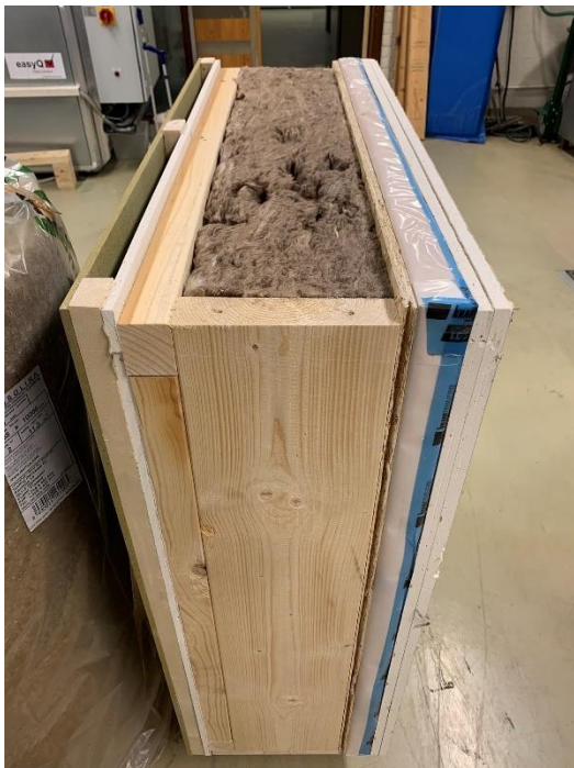
Figure 3: Mineral wool inside one of the elements.
