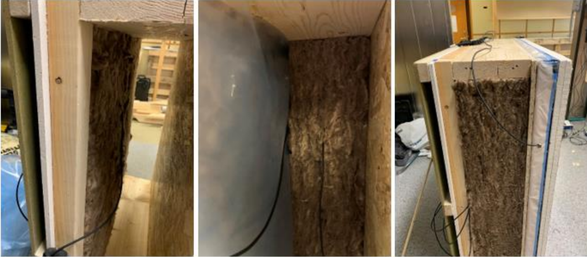
Figure 19: Actual location of Onset S-THC-M008 sensors. (a) left, (b) middle, (c) right.
