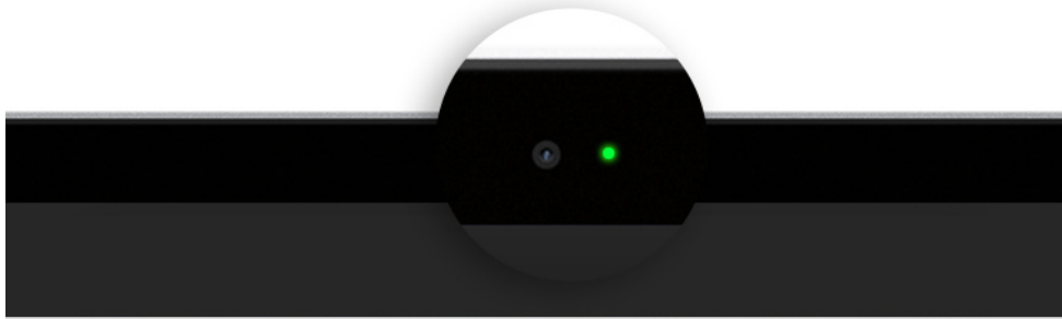
FIG. 2 Hardware solution implemented on a Macbook Air to signal camera usage (Apple, 2022)
