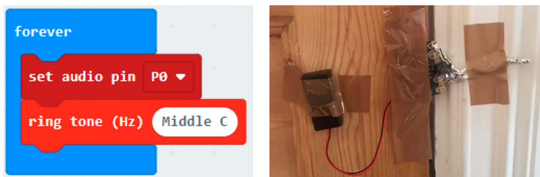
Figure 3. Visual (digital) artifact (left) with a micro:bit (right) for controlling audio in a simple burglar alarm.
