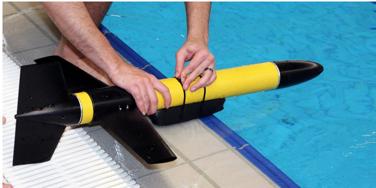
Figure 1.1: OASYS underwater glider, courtesy of Oslomet
