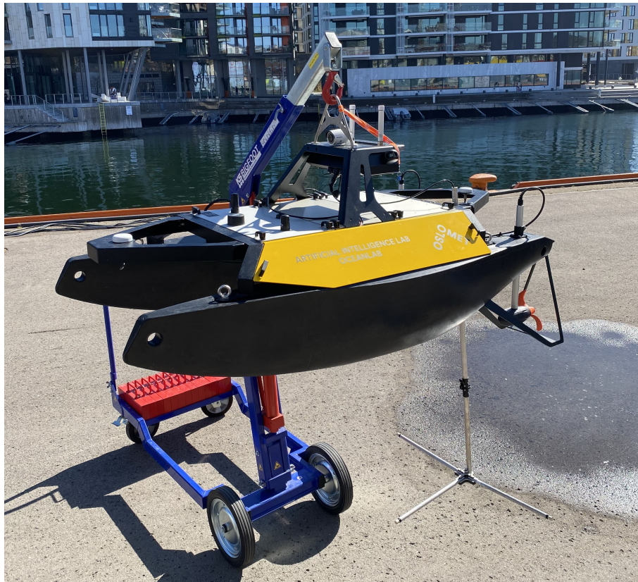
Figure 5.8: Oceanlab's Otter USV equipped with Waterlinked SBL (short baseline) acoustic positioning system, courtesy of OsloMet
