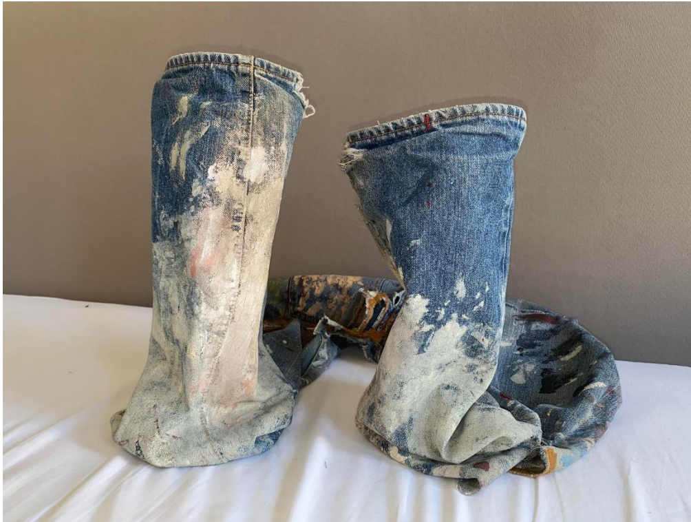
Figure 5. Image showing how the lower jean legs can stand upright without support, due to the stiffness induced by the paint stains.
