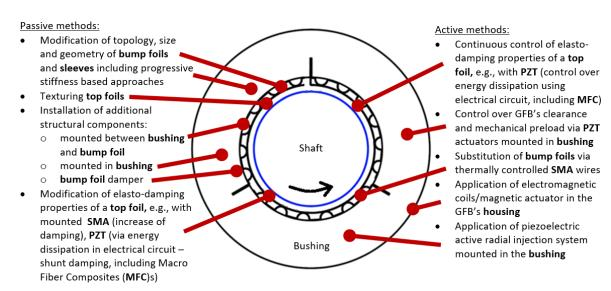
**Figure 2.** Scope of structural modifications in GFBs introduced to enhance the elasto-damping properties of the bearings. Various topology, size and geometric changes may be taken into account to improve the performance of GFBs. The modifications may affect both the bushing and specialized foils. Moreover, additional components (also made of smart materials) may be used to achieve an advantageous change in the bearing's properties.
