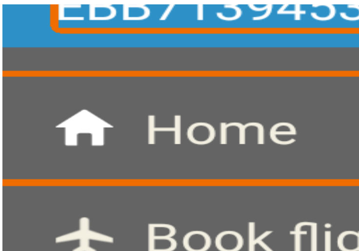
Illustration 17: A touchable button having size less than 48dp by 48dp in the SAS application
