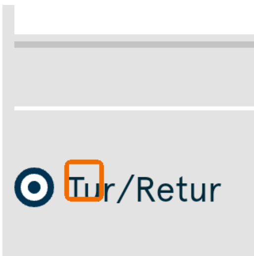
Illustration 3: A checkbox with size less than 48dp by 48dp
