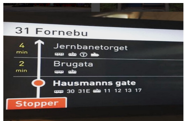
Fig. 2. Display screen showing upcoming stops and estimated arrival time in public buses.
