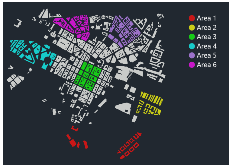
Figure 4-8. The six areas of the Downtown-model. Wind direction is from the bottom to the top
