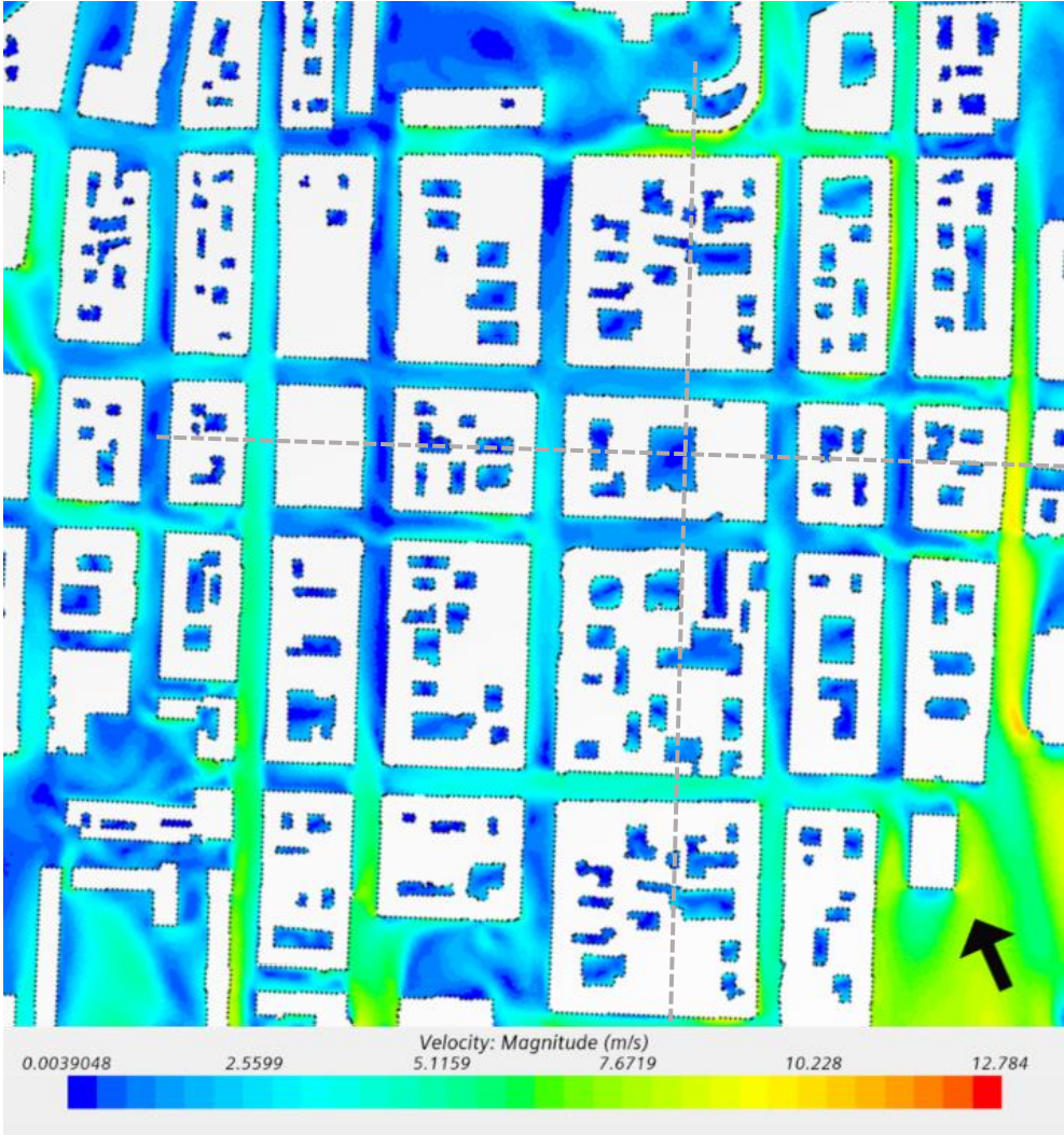
Figure 4-25. Wind velocity for Area 3, up to 17m. The dotted lines show the placement of planes for the vorticity results
