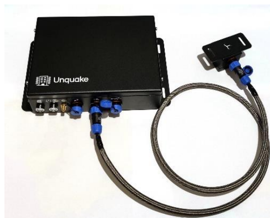
Figure 18. Unquake sensor and datalogger setup [52].
