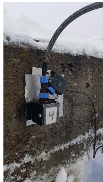
Figure B.3. Accelerometer and GPS unit setup.
