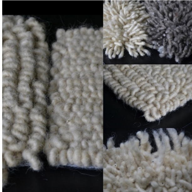
Figure 1-3: Some results of tufting tests done by our Polish partners with yarn made at Selbu spinning mill from wool of Polish Mountain Sheep (photos: private).
