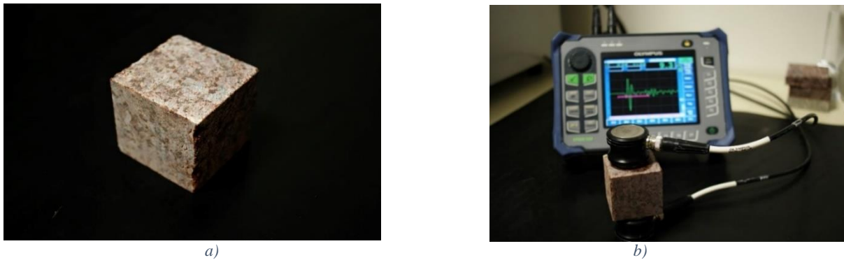
Figure 14 a) Masonry syenite stone samples, b) EPOCH650 ® ultrasonic flaw detector (olympus)
