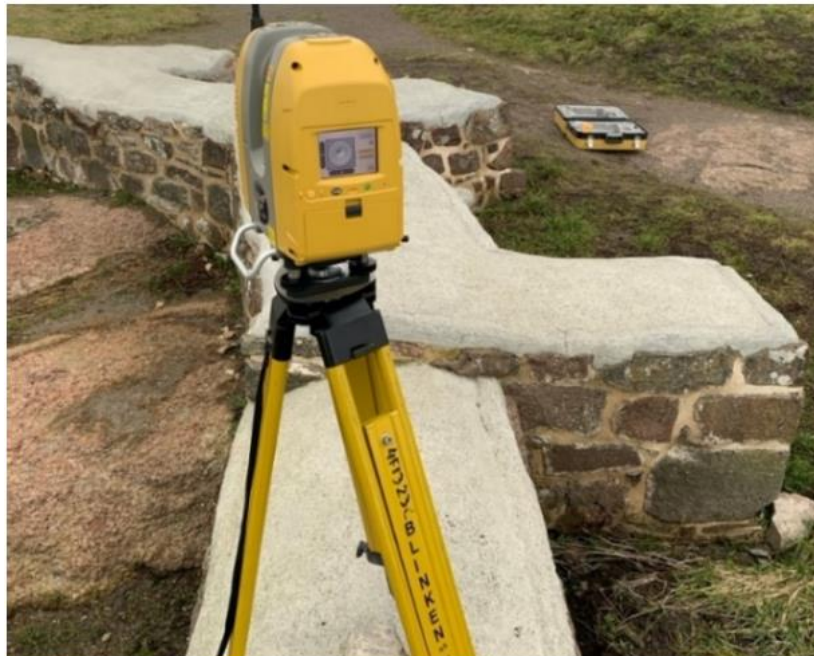
Figure 6 3D laser scanner calibrated on the outside of the Slottsfjell tower [1]
