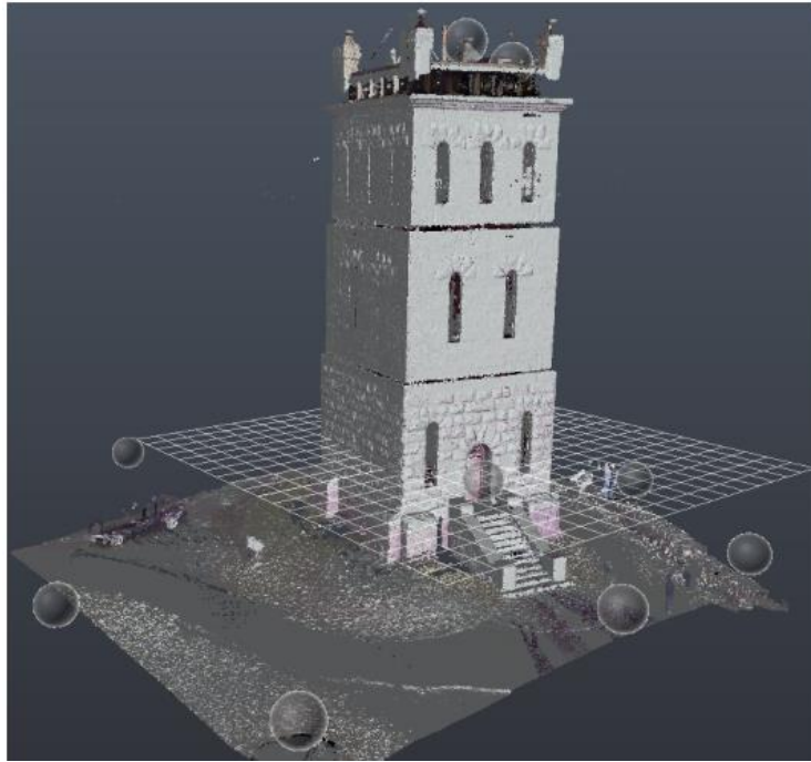
Figure 7 3D model of the Slotts fjell tower in Recap [1]
