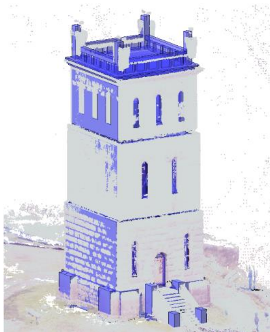
Figure 8 Point clouds imported from Recap into Revit [1]
