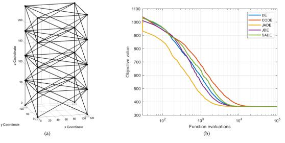
Fig. 3. (a) The 72-member space truss (coordinates in inches), (b) Convergence history for the 72-member space truss example.
