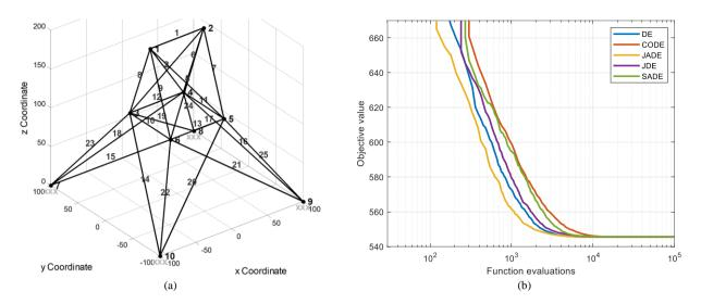
Fig. 2. (a) The 25-member space truss (coordinates in inches), (b) Convergence history for the 25-member space truss example.
