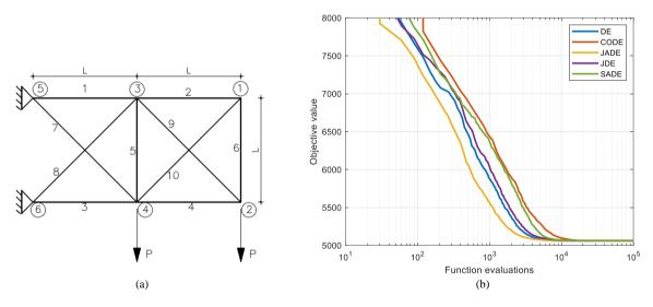
Fig. 1. (a) The 10-bar plane truss (coordinates in inches), (b) Convergence history for the 10-bar plane truss example.
