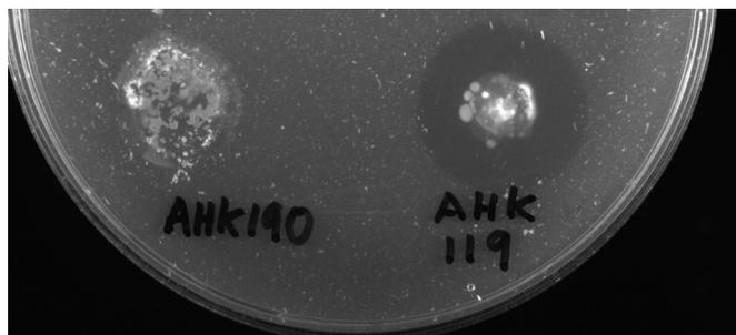
**Fig. 3.** After incubation of *S. viridis* (AHK190) and *T. alba* (AHK119) for two weeks on PET-agar (50 °C) a few grains of PCL were sprinkled on the plate in the vicinity of the growth, and plates were re-incubated for a further 3 days. A zone of clearing in the PET-agar, indicating PET hydrolase activity, was obtained with AHK119 and *T. fusca* DSM 43793 (result not shown), but not with *S. viridis* (AHK190).
