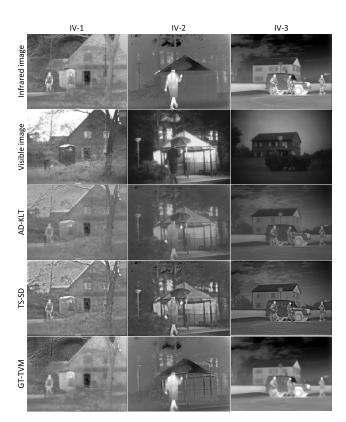
FIGURE 8. Fusion results on infrared-visible image pairs.
