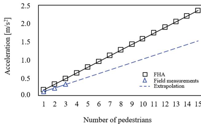
Figure 9: Measured and computed maximum accelerations for Kjærø Bridge
