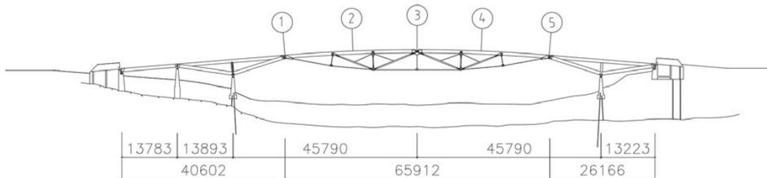
Figure 2: Elevation view: Kjærra Bridge with points of measurements (all dimensions in mm)
