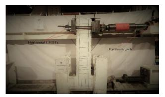
Figure 1. Laboratory setup of the beam-column joints [8]
