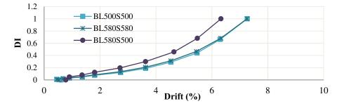
Figure 2. Displacement-based damage indices of the beam-column connections
