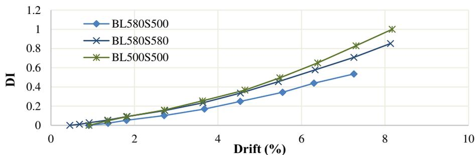
**Figure 3.** The energetic damage indices of the beam-column connections
