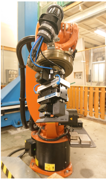
Fig. 9. KR16 ready to transfer the stapler.
