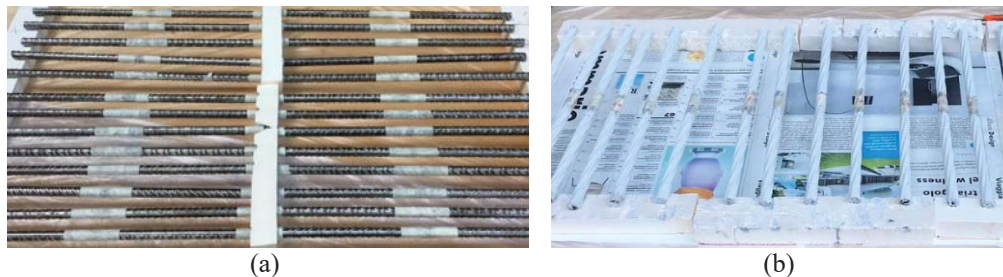
FIGURE 1. Superficial treatment of the bar: (a) ribbed reinforcement after cleaning, (b) steel strand after the antirust application.
