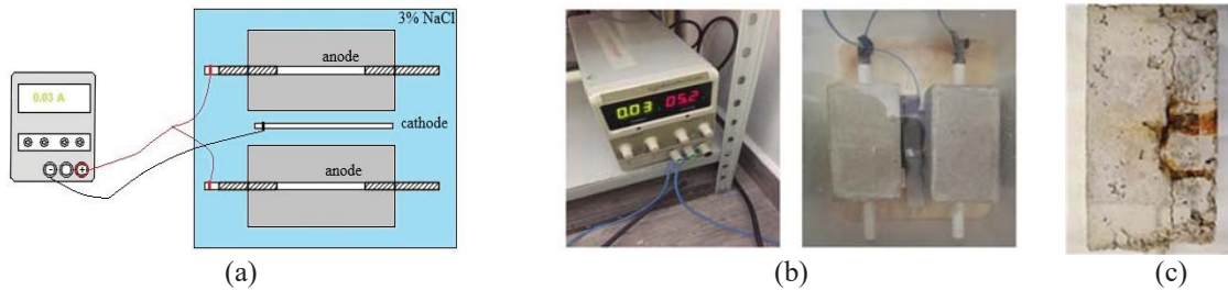
FIGURE 4. Preliminary corrosion test on c/d = 3.67 bond specimens: (a) schematic illustration of the procedure, (b) accelerated corrosion test setup in the laboratory, (c) crack pattern after 12 days.
