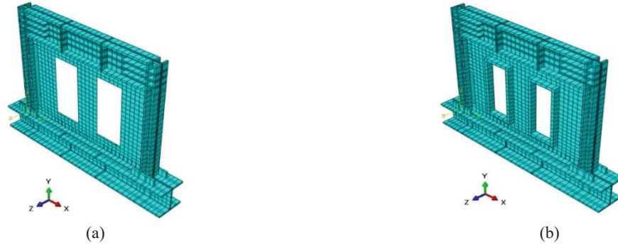
FIGURE 3. Mesh sizes of the FE models: (a) NS-SPSW without stiffener, (b) OS-SPSW with stiffeners around the openings.
